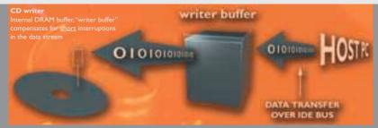
Fig. 2, Typical CD writing process: Short interruptions in the transfer of the data over the IDE bus will cause the writer buffer level to drop.
